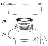
Turn the locking ring with cutting assembly (c) upside down, and place the blade end in the blender jar opening. Engage threads by twisting the locking ring clockwise until tightened. Make sure locking ring is tightly fastened to blender jar. Once assembled, turn the blender jar right-side up.
